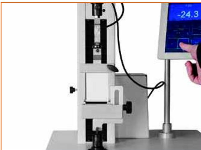
Sample support for the Wet Tensile Strength Test (Finch)
