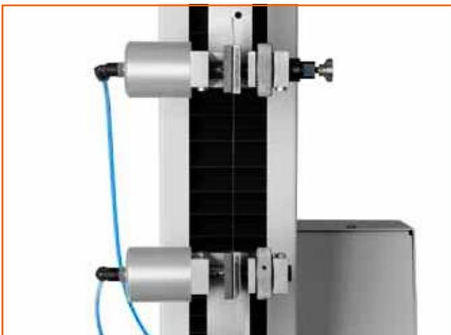
Pneumatic clamps for the Dry Tensile Strength Test
