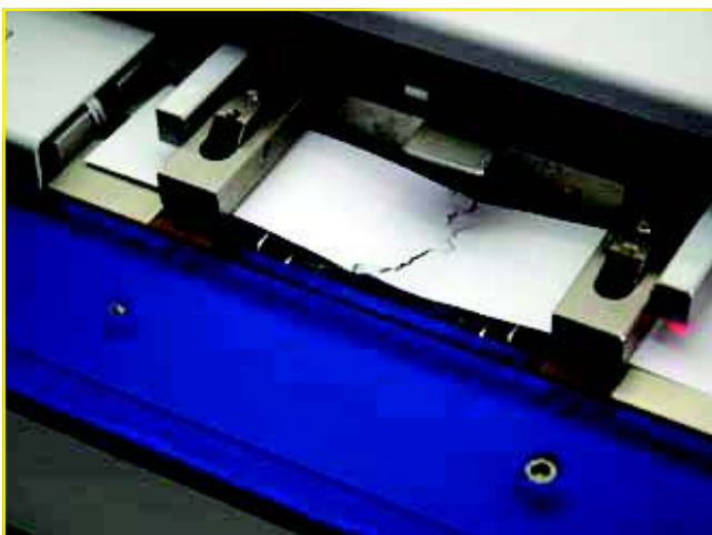
The sample is lifted out of the water and stretched till it breaks
