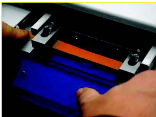
A sample with a width of 15 mm is placed between the test clamps
