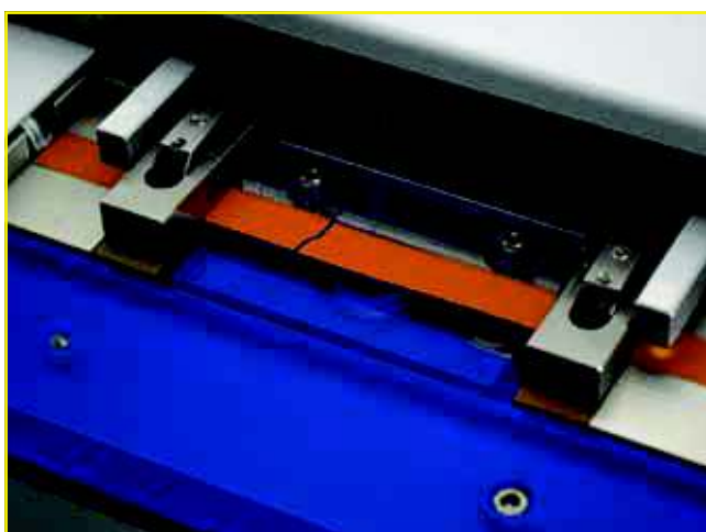
The sample is stretched till it breaks
