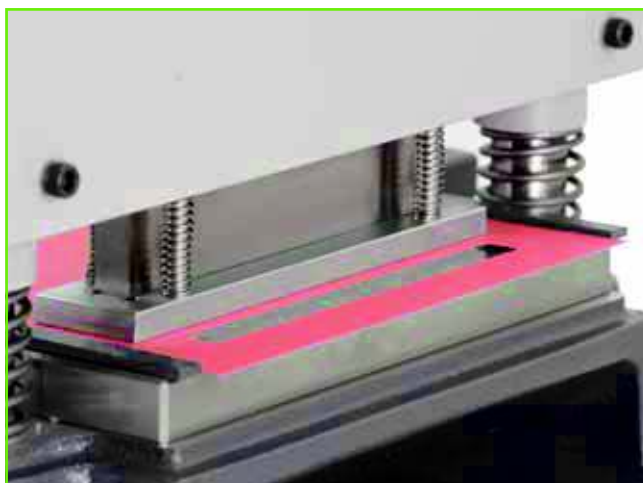
A clamping mechanism holds the sample during punching
