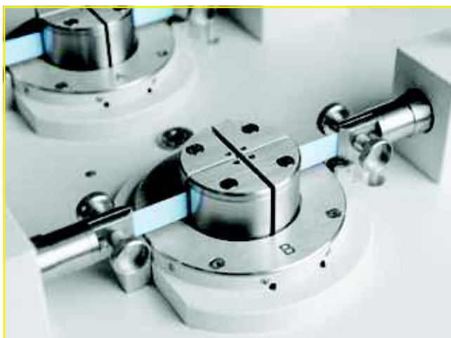
The samples are clamped with spring-loaded sample carriers
