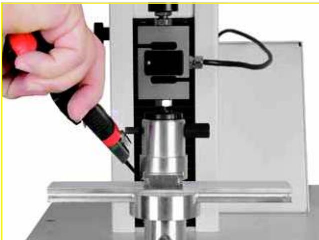
The sample is cut with a sharp knife to the left and right
