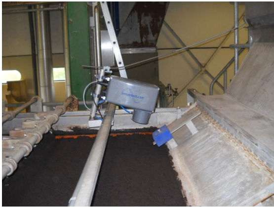
On-line NIR moisture meter for measuring moisture in sludge from waste water
