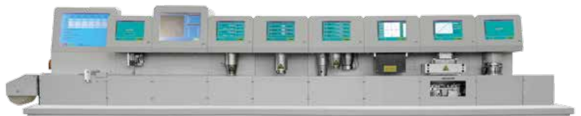
Testline for various measurements like colour, thickness, smoothness, roughness, tensile, base weight, moisture etc.
